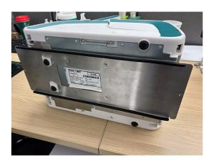
2. Attach the mounting plate to the SLS PCS with the four supplied thumbscrews.
