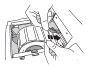
5. Place the label media below the media guides and into the feeder slot.
