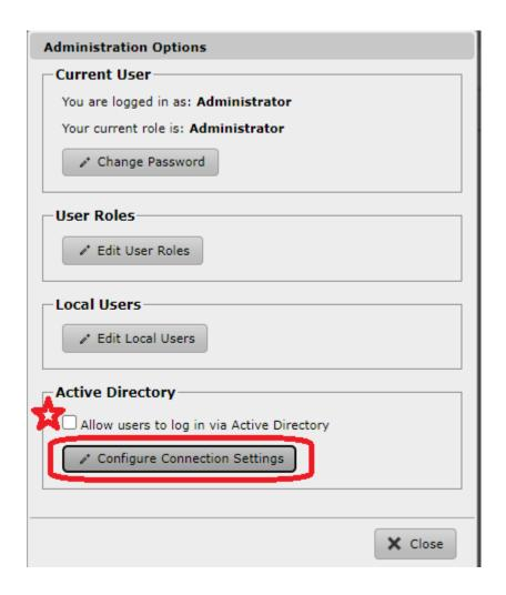
v. Enter the AD settings into the "Configure Active Directory Settings" dialog. Check "Use SSL" and change the Port setting to the appropriate SSL port (636 is typical).
