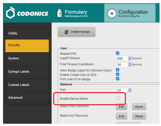
iv. Uncheck "Enable Device Name" under the "Network" section.
