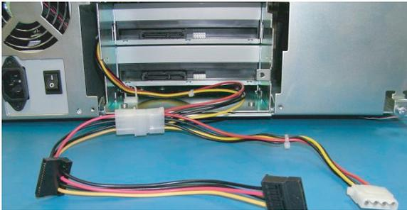
3. Mark the location of the drive bay bracket on the chassis using a felt-tip pen at the front of the Recorder as shown.
