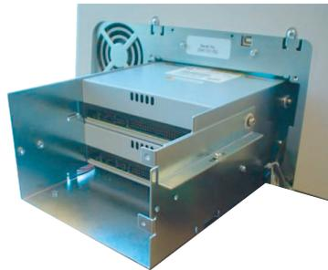
**NOTE:** Use care when removing the drive bay, the power supply cables are easily pinched.
