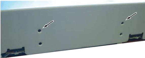
8. Reinstall the drive bay. Align the drive bay bracket to the mark made in step 3. Using the two short screws and two washers, secure the front of the drive bay. Use the Torx driver to torque both screws to approximately 6 in-lbs (0.68 Nm).
