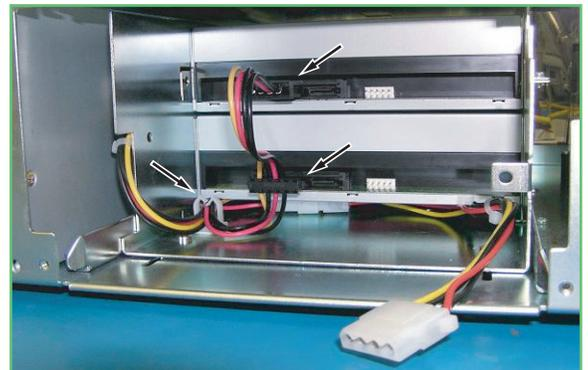
11. From the fan assembly, plug the SATA cable that is closest to the center of the Recorder into the upper optical drive. Plug the remaining SATA cable into the lower optical drive. Plug the drive bay fan into the remaining drive power connector in the bay. Use the Torx driver to secure the fan assembly with four screws. Torque the screws to approximately 6 in-lbs (0.68 Nm).
