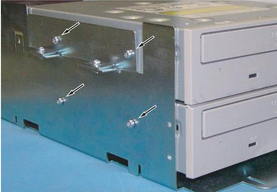
**NOTE:** Do not remove the two screws holding the two top optical drive mounting brackets. If the top drive needs to be adjusted for calibration, loosen the two screws holding the two top optical drive mounting brackets. Adjust position and tighten screws to approximately 6 in-lbs (0.68 Nm).
