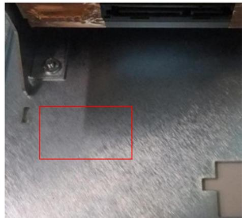
3. Place a cable tie mount on the drive bay. The left edge of the cable tie mount should be aligned with the center of the bracket fastener and 5/8 of an inch below as shown in the following image.
