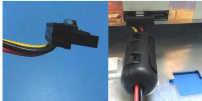
7. Seat the ferrite on the exposed adhesive on top of the cable mount.
