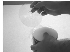
3. Properly take a handful of discs, and loosen them, as shown below. Place the discs on the spindle of the disc holder making sure the white surface is facing up.
