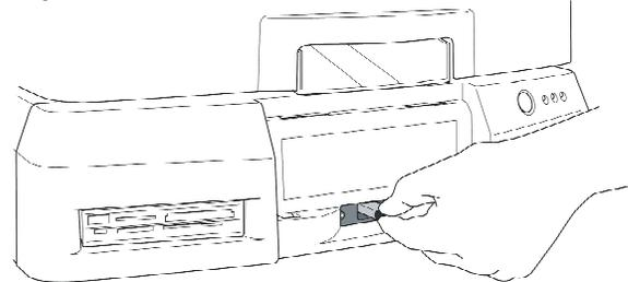
3. Connect the SmartDrive to the USB port of the PC.
