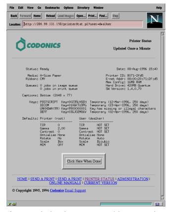
This section displays the current status of the printer and user settings. It is a single page which automatically updates once per minute. The output is similar to the **stat** command.
