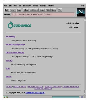
Configures and administers the printer. All major printer functions, including Security and Accounting, Network Configuration, and Default Image Settings are controlled through this section. Access to this section of ImageWeb requires the printer's root password.
