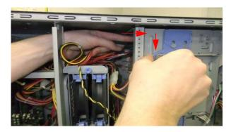
7. Push up the blue colored lever for preparation of installing the new Blu-Ray drive.
