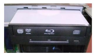
9. Install the Blu-Ray drive by inserting it into the front panel slot and pushing it back until it locks into place.
