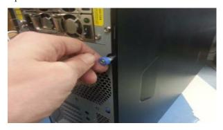
3. Gently lift the three black colored clips holding the front panel and swing it fully open to the right side.
