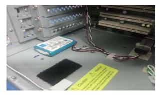
4. Carefully unplug the RAID battery from the underside of the RAID controller card. The female end slides back (toward the motherboard) to release.
