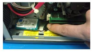
3. Place the new battery on the velcro pad and reconnect the new battery.
