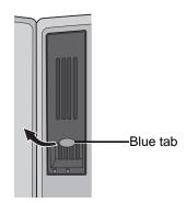
Slide the hard drive out of the old chassis.
