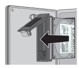
**CAUTION:** Use care when handling hard drives. Do not drop the hard drive. Handle only the front, side edges, and face with the label. Do not handle the underside or the backplane of the drive. Do not touch any exposed electronics.
